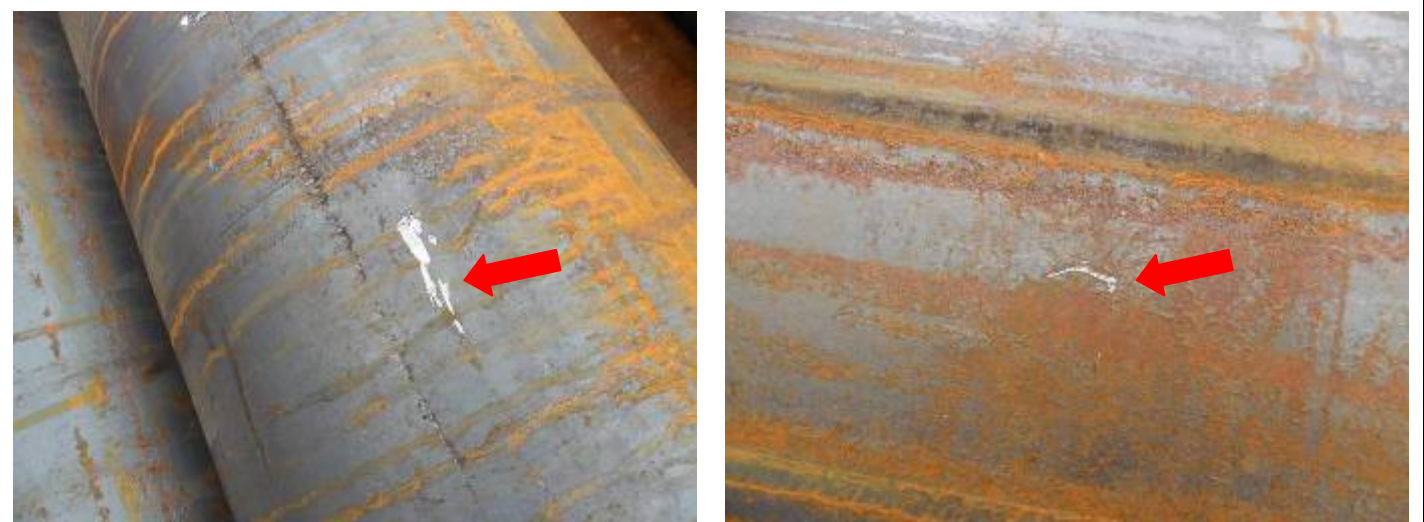
Minor : Few oxide films on outer surface. -2pcs
