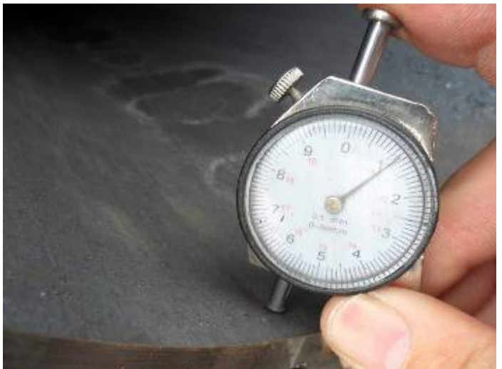
26. Wall thickness test : 10.6mm
