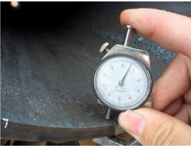
29. Wall thickness test :10.6mm
