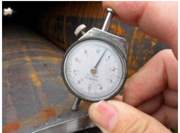
28. Wall thickness test : 10.5mm
