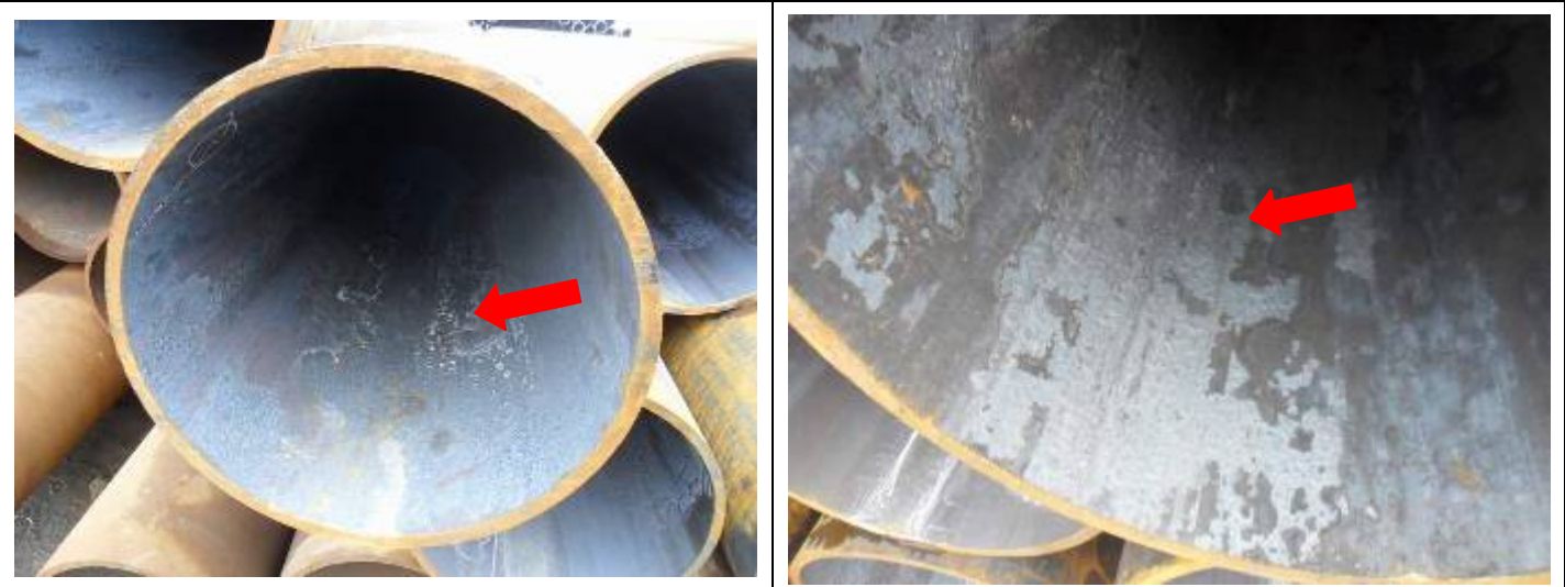
Found there are many oxide films on inside surface. Required the factory should clear these oxide films before the inside surface is coated the epoxy resin paint.
