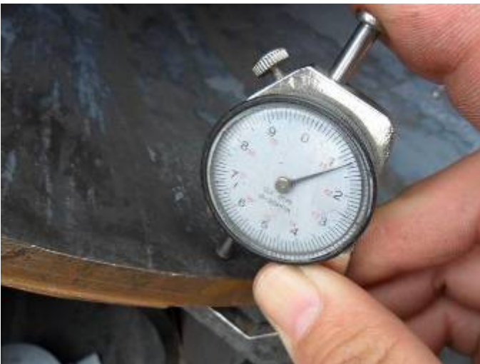
23. Wall thickness test : 11.3mm
