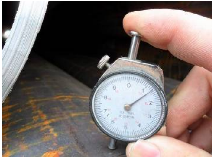
30. Wall thickness test :11.3mm
