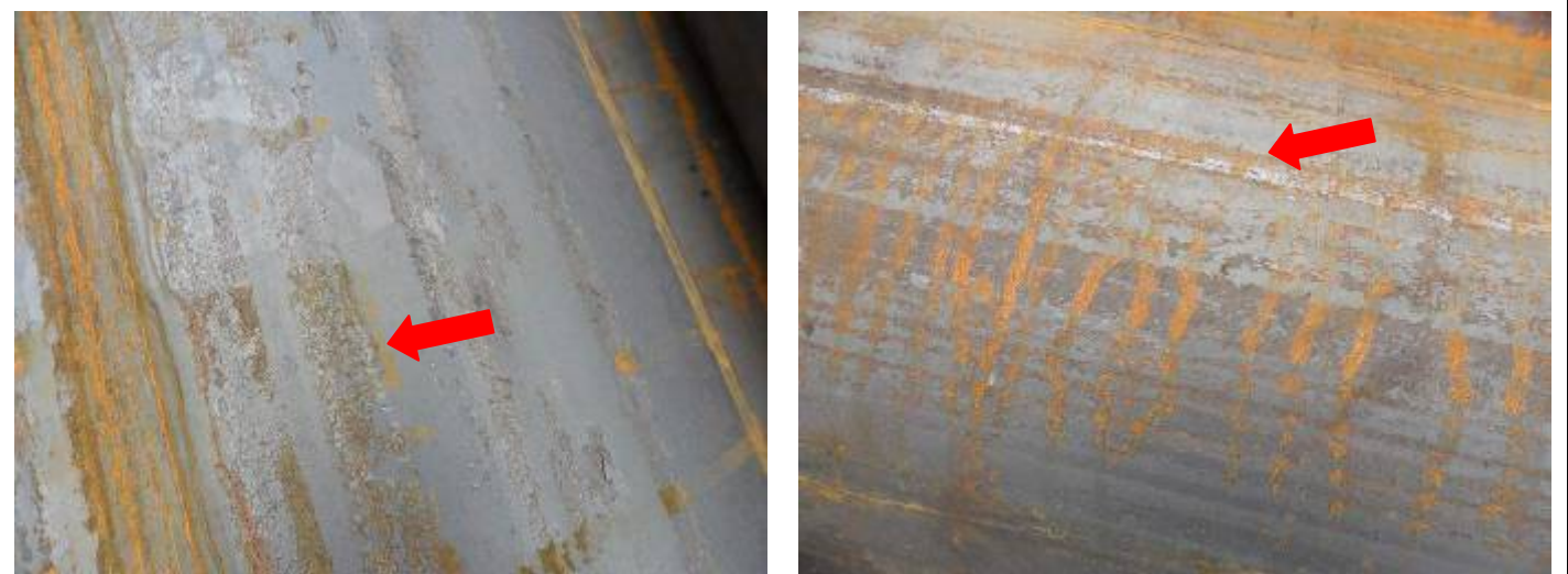
Minor : Few oxide films on outer surface. -2pcs
